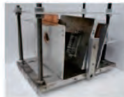
Figure C.4 — Picture of target and witness plate set-up for oblique impact (Front witness plate can be removed when the front ejecta is negligible.)
