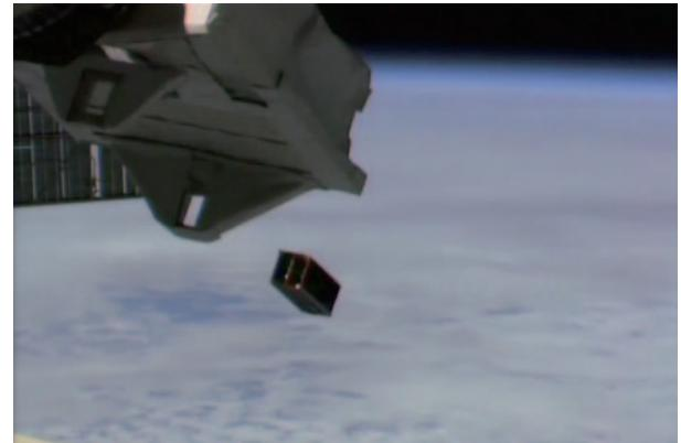
Figure 2. SPATIUM-I satellite release from the ISS
